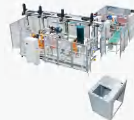
抽油烟机箱体铆接生产线 Automatic Clinch Machine For Range Hood
