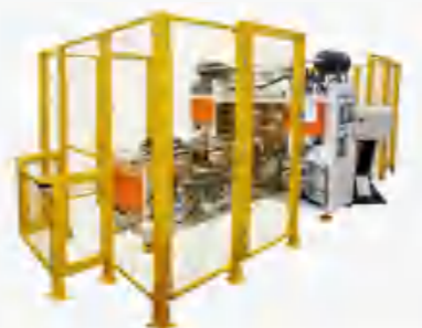
440KVA 货架顶底板长边加强筋中频焊机 440KVA MFDC Multi Spot Welder For Supermarket Shelf
