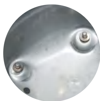
压簧支柱焊接 Welding Of Pins
